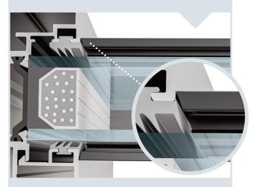
For cross over joints a 4 degree cut will reduce the chance of the bar end showing.
