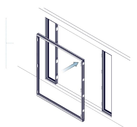
Do not drill into gasket chamber
