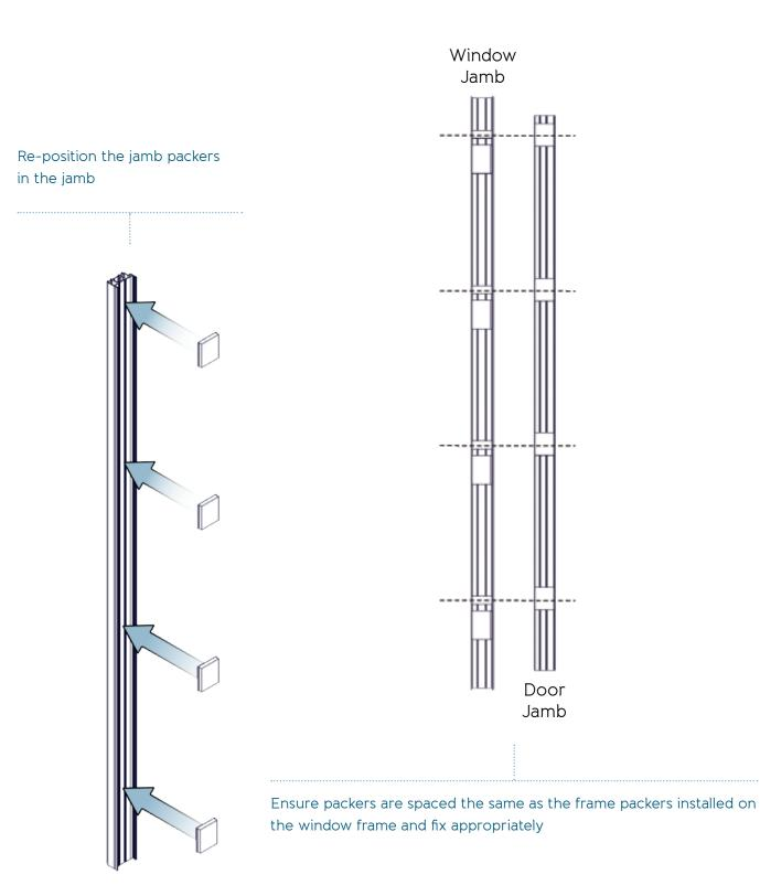
Position the door frame into the aperture and pack/ clamp accordingly
