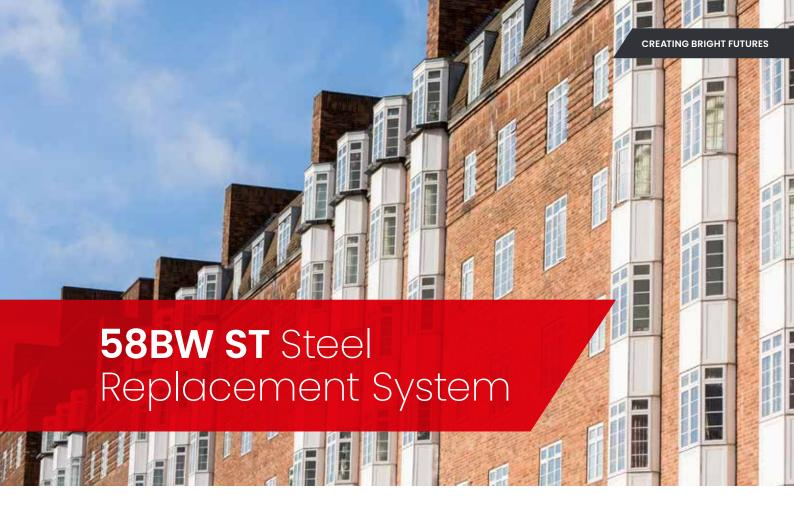
Ideal for projects where planning or design requires the installation of sympathetic materials, our 58BW ST Steel Replacement Window System provides the look of steel with the benefits of aluminium. Designed to replace and complement existing steel windows, the range has been specifically developed for use on listed buildings, warehouses and similar buildings, where steel windows have always traditionally been fitted.
